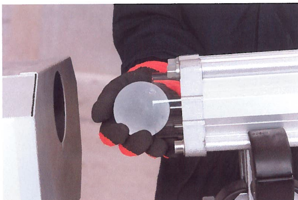
Illustration 2: loading of the equipment, with a laboratory made, transparent, ice ball (70 mm diameter)
